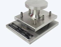
The device is designed to perform PV 3307 deformability test on 6 rubber or plastic samples with a diameter of 15 mm and a thickness of 2 mm.
