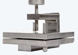
The device is designed for the testing of the permanent deformation of finished parts and O-rings according to PV 3330 method. **Key Features**
